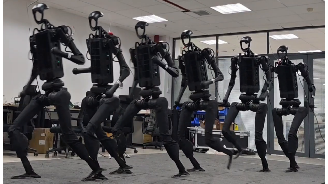
Fig. 1. Gait pattern transitions during forward velocity ( v_x ) acceleration from 0.7 m/s to 1.8 m/s
